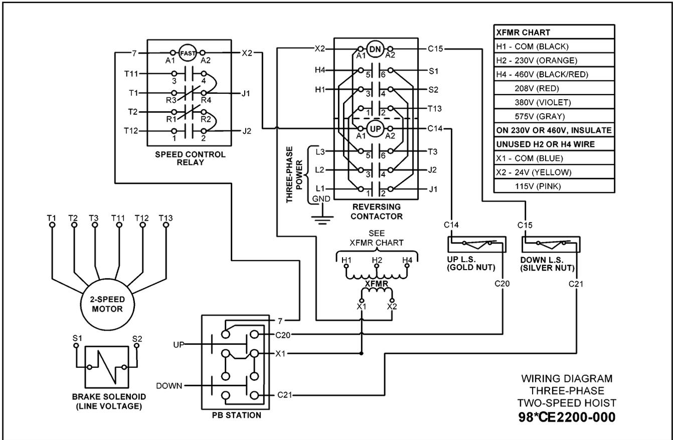
**Figure 9D — Wiring Diagram for 2-Speed, 3 Phase Models**
