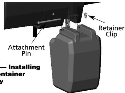
**Figure 1 — Installing Chain Container Assembly**
